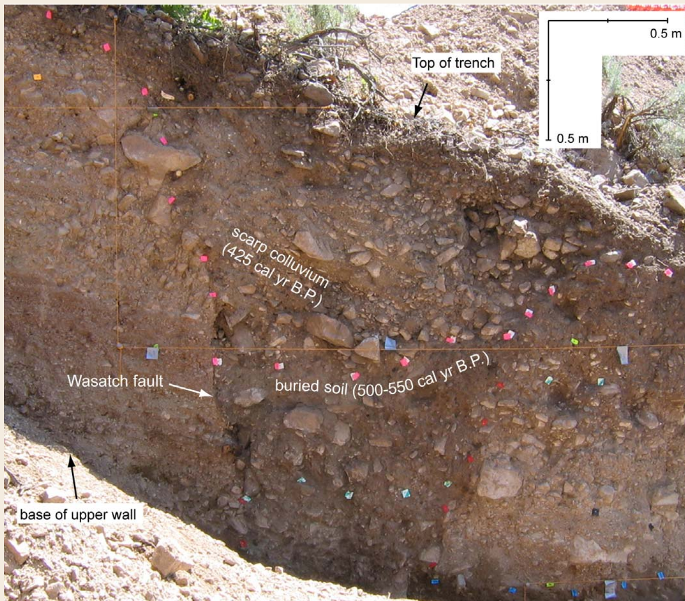
Figure 2. Santaquin trench exposure, showing soil displaced along the Wasatch fault (white arrow) and buried by scarp colluvium (above pink flagging). Horizontal level lines (orange) and 1 meter apart.
