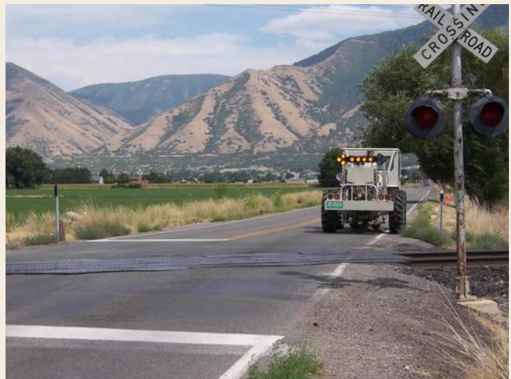
USGS minivibe working along Utah State Highway 147 between Spanish Fork and Mapleton.
