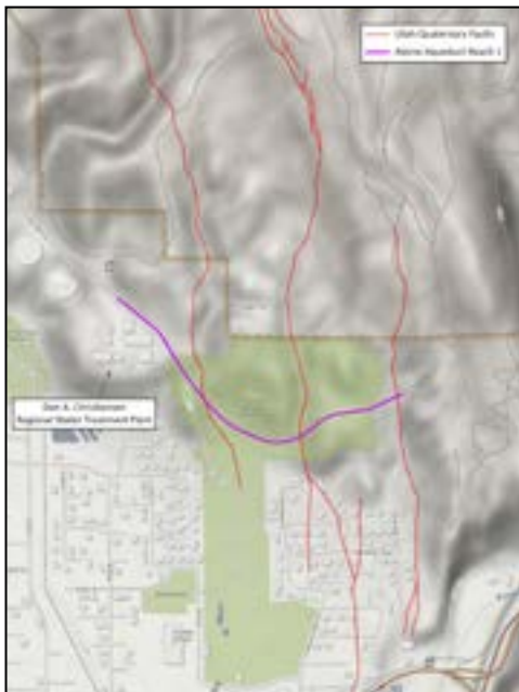
The Alpine Aqueduct (purple) crosses faults (red) in multiple locations as well as a known landslide area.
