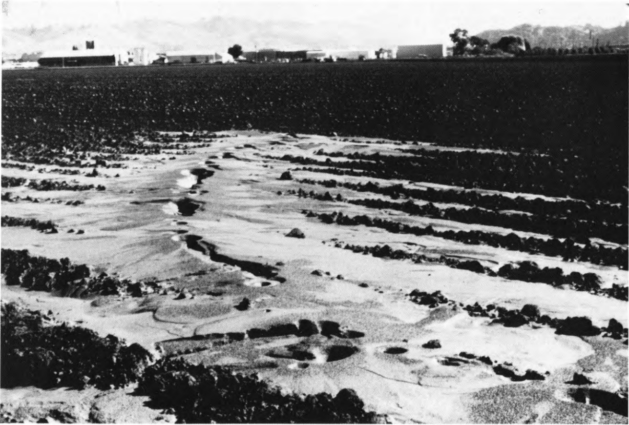
Figure 29. Sand boils in irrigated fields near Hollister.
