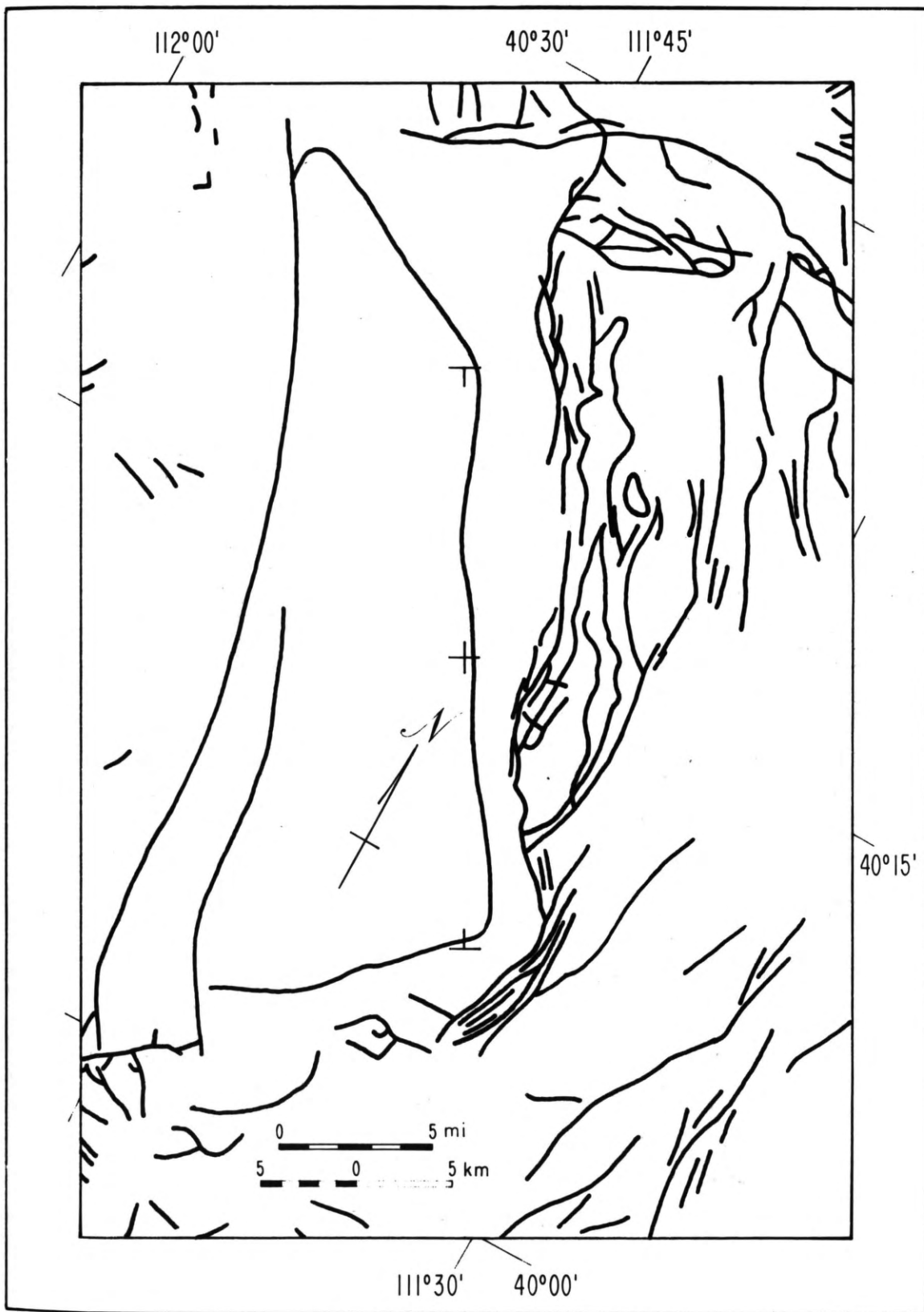
Figure 16.--Area of probable faulting for the Provo close-in event. + indicates the assumed epicenter; ┐ and └ indicate the ends of the assumed fault.
