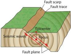
The above diagram shows an earthquake that starts underground and ruptures along an inclined fault, and some earthquake terminology. During earthquakes of magnitude 5 and larger, the earthquake rupture may continue all the way to the surface, creating visible offsets of the ground. [Referenced from <u>http://ykonline.</u> <u>yksd.com/distanceedcourses/Courses/EarthScience/lessons/</u> FourthQuarter/Chapter13/13-04/Images/focus.GIF.]
