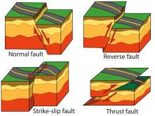
These diagrams show different kinds of fault movement that can occur during earthquakes and a geologist may use these terms. (Referenced from <u>http://soundwaves.usgs.gov/2009/11/fieldwork2.html</u>.)
